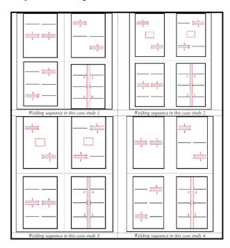
Figure 5: Welding sequences in the case study 1 to 4.
