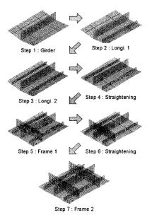
Figure: Welding deformation of each assembly stage
