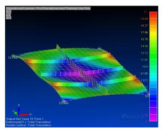
Figure 10: The computational result of total deformation. [1]
