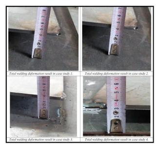
Figure 6: Total welding deformation result from case study 1-4.
