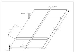
Figure 3: CAD Model with a base plate, one longitudinal flat bar and three transverse flat bars.
