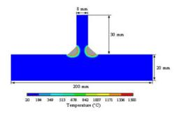
Figure 2: T-fillet welding performed to analysis thermal conditions in the thin plate. [5]
